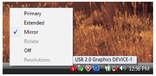
the secondary CRT/LCD monitor. The screen resolution setting on the secondary monitor will follow the primary screen's resolution. If the selected resolution setting is not supported by the primary screen, however, a warning dialog box will be displayed and the suggested screen resolution will be shown.
